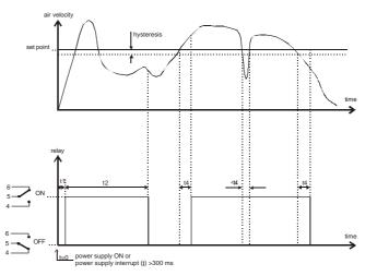
Only after that the air velocity switch reacts to the TRUE and RATED VALUE. The reaction time is limited by the response time ( $t_4$ ) of the sensor probe which is about 2 s. The described function is related to continous operation, which is reached after a warm-up phase of approx. 3 min after applying the supply voltage.
